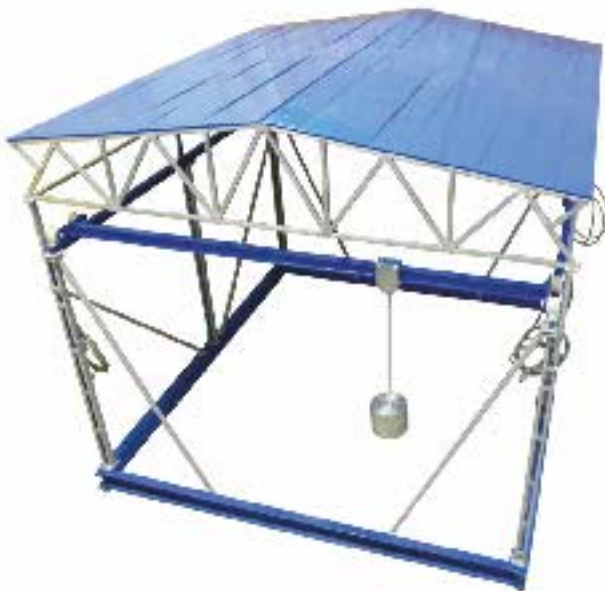
Industrial building load-bearing structures model
