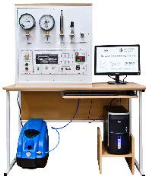
Automatic pressure control and management systems (ACS-D-SC)
