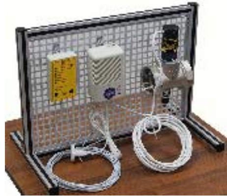
Gas pollution control system, training stand
