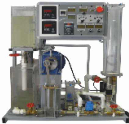
Automation of a pumping station with a piston pump (ANS-PN-6LR-10-01)
