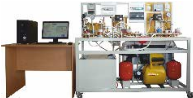
Automated heating unit (ATP-01)
