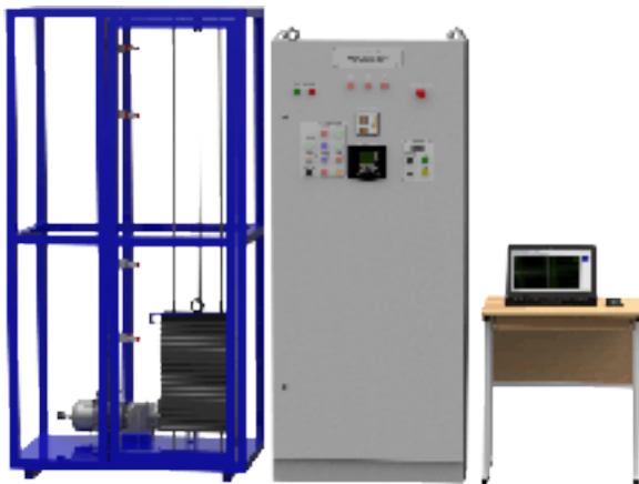
Electric crane equipment (EO-PK-ShN)
