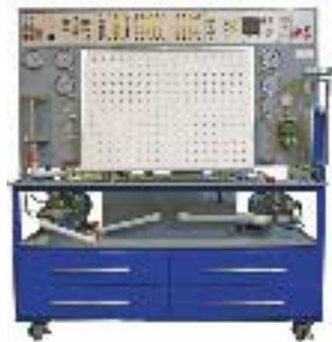
Operation and adjustment of hydraulic equipment with adjustable pumps and proportional equipment (SGU-UN-015-35LR-01)
