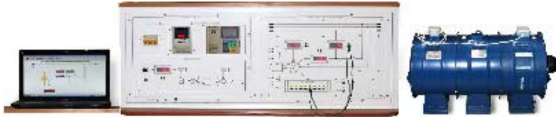
Wind power system based on an asynchronous generator operating in the grid (VES-AG-NN)
