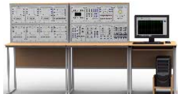
Relay protection (RZ-NN)
