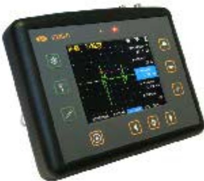
Ultrasonic control of polyethylene pipes
