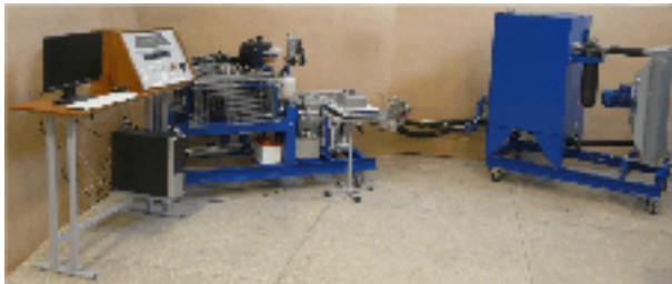
Operating processes of a 4-cylinder gasoline/diesel engine with a motor-generator or hydraulic loading unit
