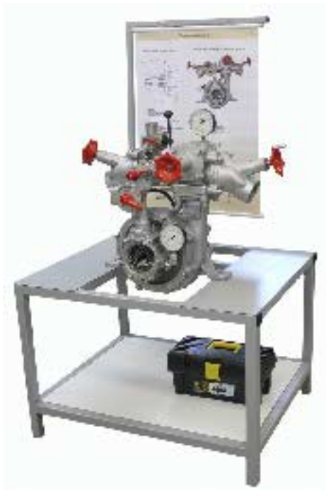
Fire Pump, training stand
