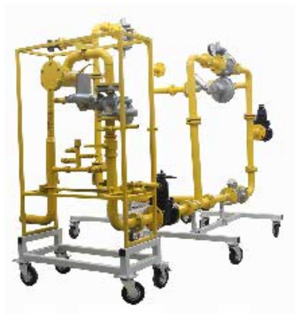
Installation of gas distribution network equipment, training stand
