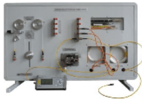
Fiber-optic communication line VOLS-02
