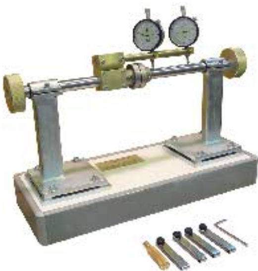
Alignment of shafts in the horizontal plane CVGP-015
