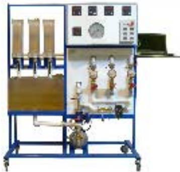
Metering and control devices in water supply systems
