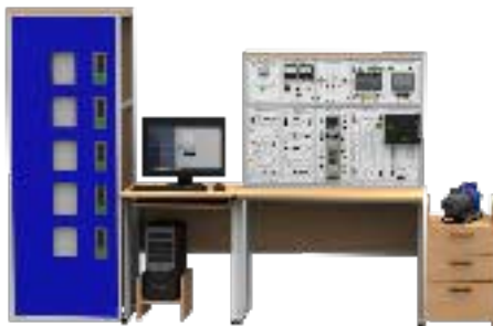
Electrical equipment and automation of the elevator (EOiA-L-SK)
