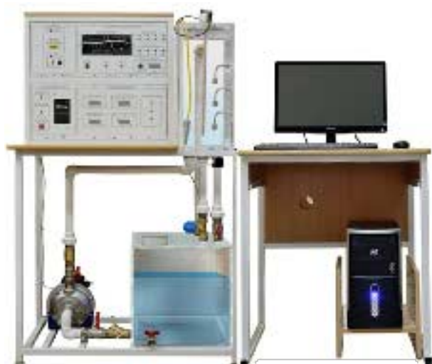
Automatic level control and management systems (ACS-U-SC)
