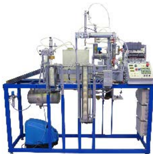
Automated liquid dosing and packaging line (AL-DUZh-13LR-01)
