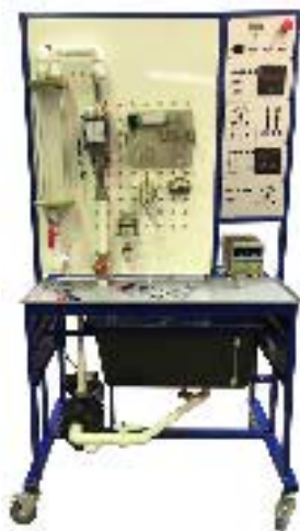
Installation and connection of hydraulic and mechanical measuring instruments (MP-KIP-GM-017-60LR)
