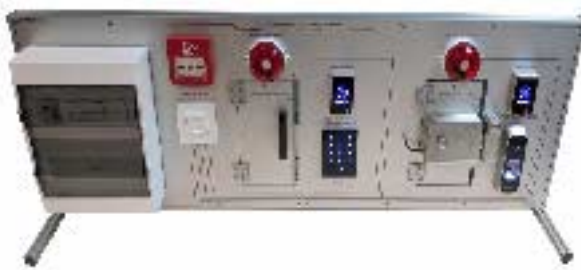
Internet of Things access control and management systems, basic configuration of IoT-SKUD
