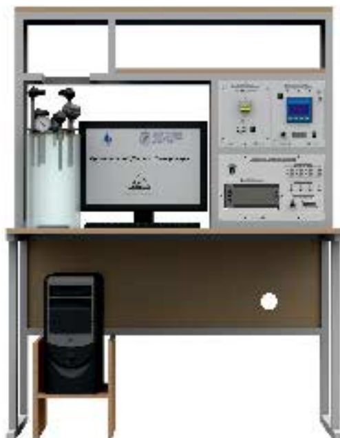
Automatic temperature control system (SAU-T-SK)
