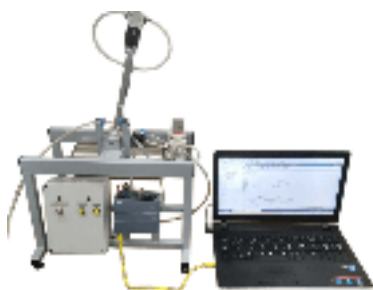
Pulsed pneumatic stabilization system (SU-IPSS-018-14LR-01-PK)
