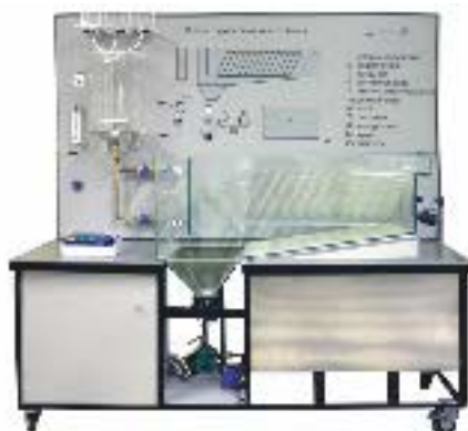
Horizontal settling tanks
