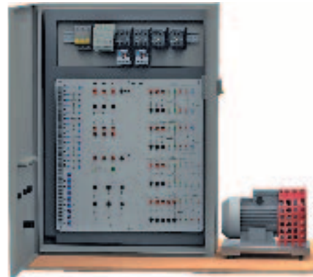
Control system of a two-speed asynchronous motor with a short-circuited rotor (SU-ADKR-NR)
