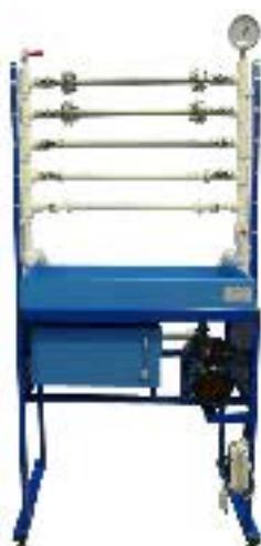
Installation and testing of pipeline connections, repair of pipelines (Mil-TS-RTr-020-4LR)
