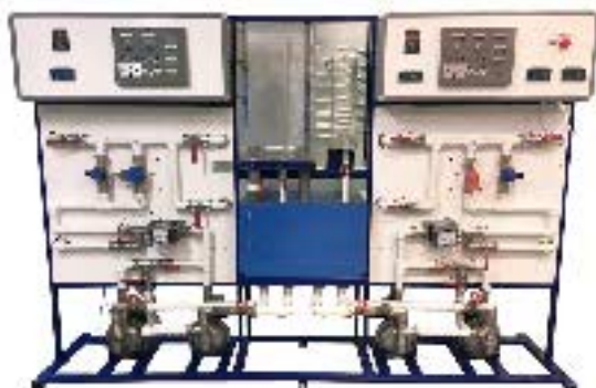
Control of the pumping station of the water supply systems
