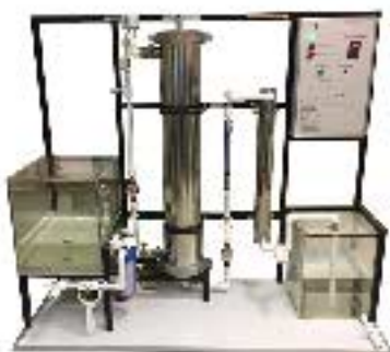
Reverse osmosis water desalination
