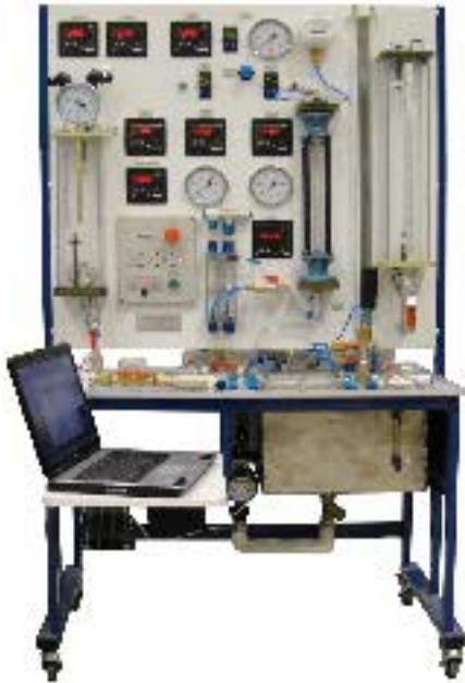
Devices for measuring pressure, flow rate, temperature and energy
