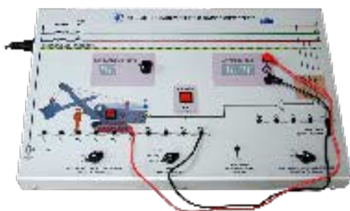
Protective grounding and self-grounding
