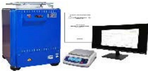
Study of the Kinetics of Alloy Oxidation in air at high temperatures
