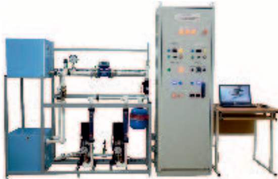
Electrical equipment and automation of the pumping station (EOiA-NU-ShN)
