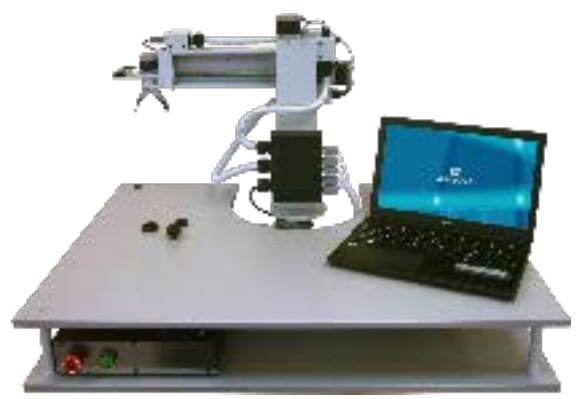
Automated assembly stand with computer control and a vision system (ARS-UR-TZ)
