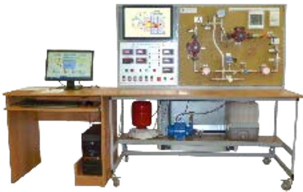
Automated gaseous fuel boiler house
