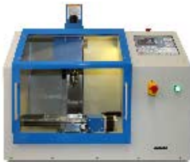
Desktop milling machine with computer control and computer simulators of turning and milling machines (UFSp-CNC-USB)
