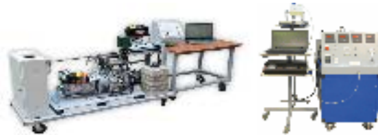
Operating processes of diesel/gasoline internal combustion engines with a motor-generator or hydraulic loading unit
