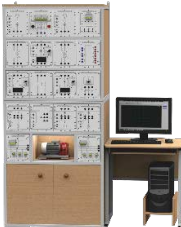
Power supply systems of industrial companies (SES-PP-SK)
