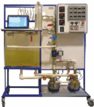
Automation of pumping stations of water supply systems (SU-ANSSV-015-17LR-01)
