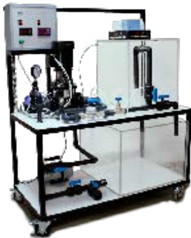
Determination of performance characteristics of a centrifugal pump
