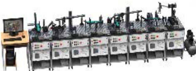
Max configuration of mechatronic devices of a sorting and assembly line (ML-PROFI-SK)
