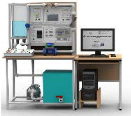
Automatic flow rate control system (SAU-R-SK)
