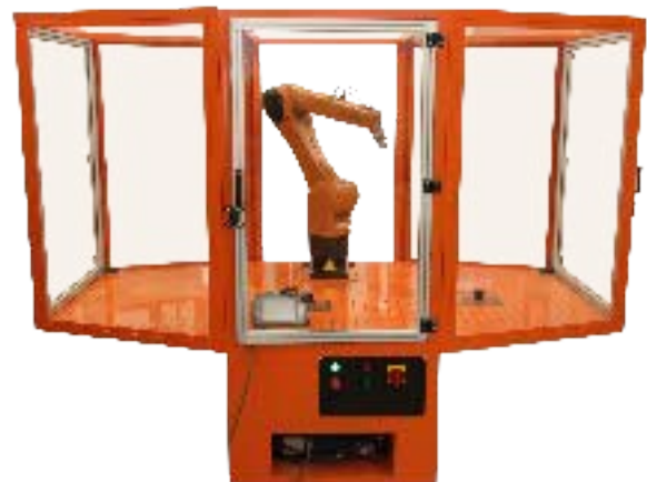
Robotic assembly cell based on the KUKA KR10 industrial robot
