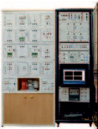
Microprocessor means of relay protection in power supply systems (MPSRZ-SES-SN)
