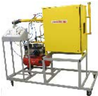
Operating processes of gas distribution point, lab stand
